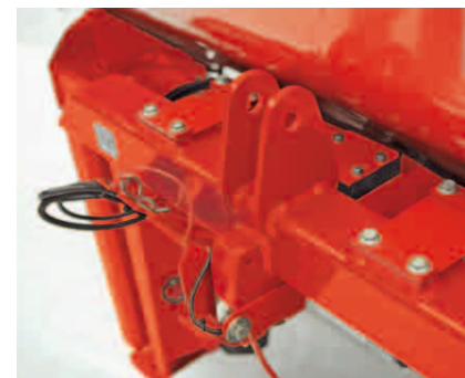
10-Tonnen Wiegezellen (Exacta CL EW)
